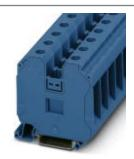
Feed-through terminal block, Connection method: Screw connection, Cross section: 1.5 mm² - 50 mm², AWG: 16 - 1/0, Width: 16 mm, Height: 65.1 mm, Color: blue, Mounting type: NS 35/7,5, NS 35/15
