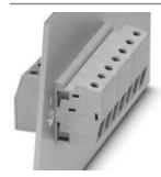
Panel feed-through terminal block, connection method: Screw connection, number of positions: 1, load current: 76 A, cross section:  $0.5 \text{ mm}^2$  -  $16 \text{ mm}^2$ , AWG 20 - 6, connection direction of the conductor to plug-in direction:  $0^{\circ}$ , width: 10.1 mm, color: gray
