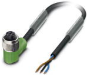
Sensor/Actuator cable, 3-position, PUR halogen-free, black-gray RAL 7021, free cable end, on Socket angled M12, A-coded, Cable length: 1.5 m
