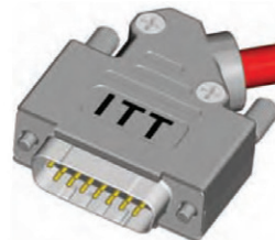
Assemble the other half (screwing force: 100-120 Ncm)
