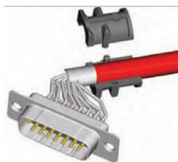
Attach the strain relief around the cable
