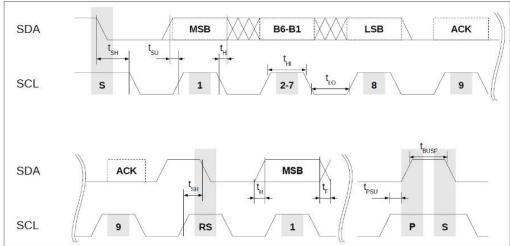
$<sup>^{\</sup>star\star}$ ) For I<sup>2</sup>C bus capacitance load >100pF maximum possible clock frequency is 100kHz
