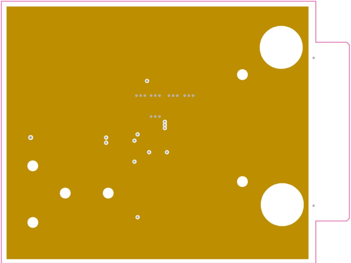
**Figure 5. Mid Layer 1 Ground Plane**
