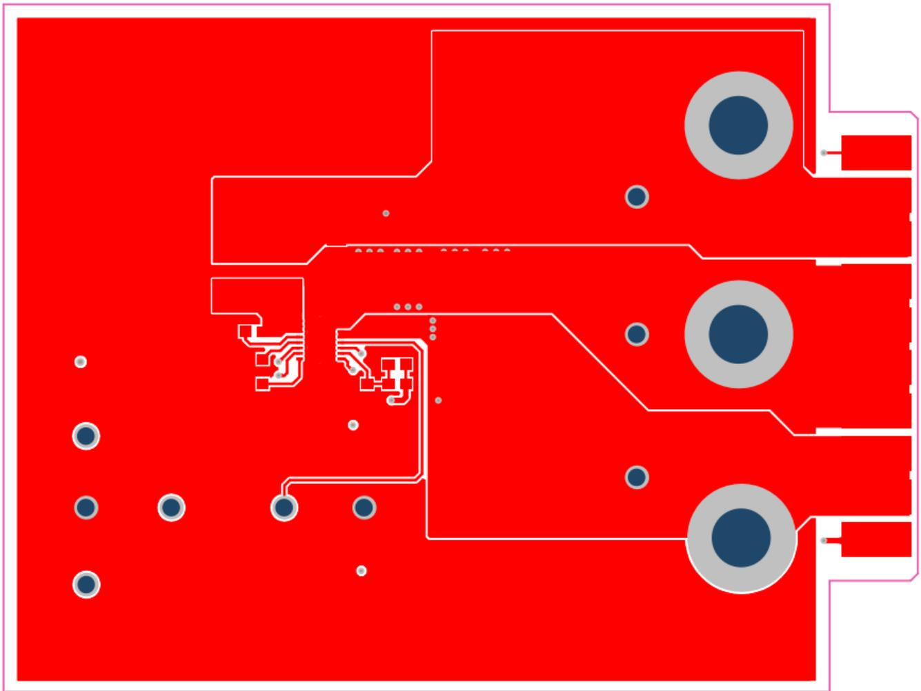
**Figure 4. Top Layer Routing**
