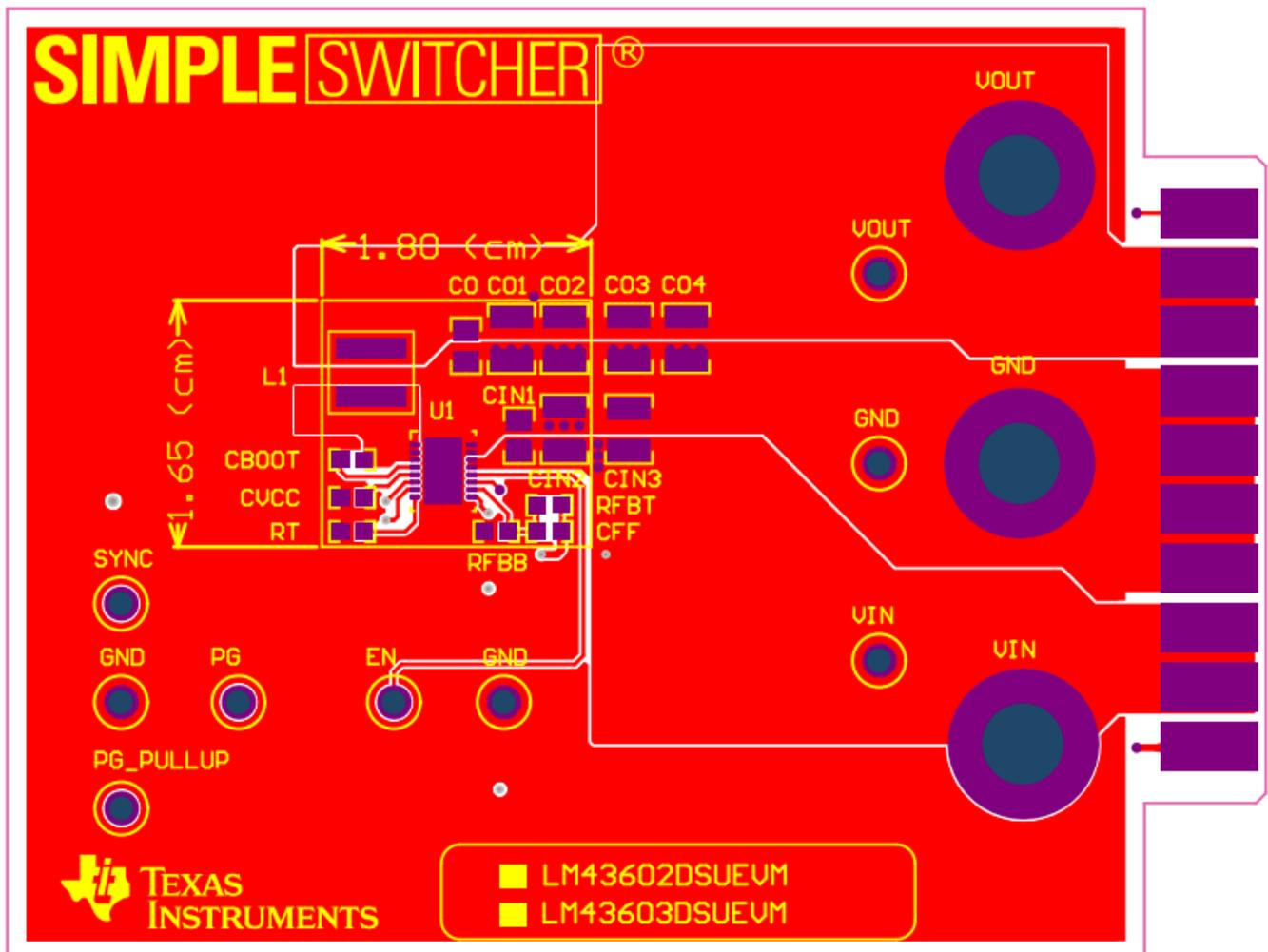
Figure 3. Top Assembly Layer
