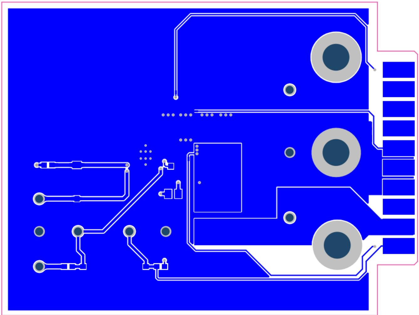
**Figure 7. Bottom Layer Routing**
