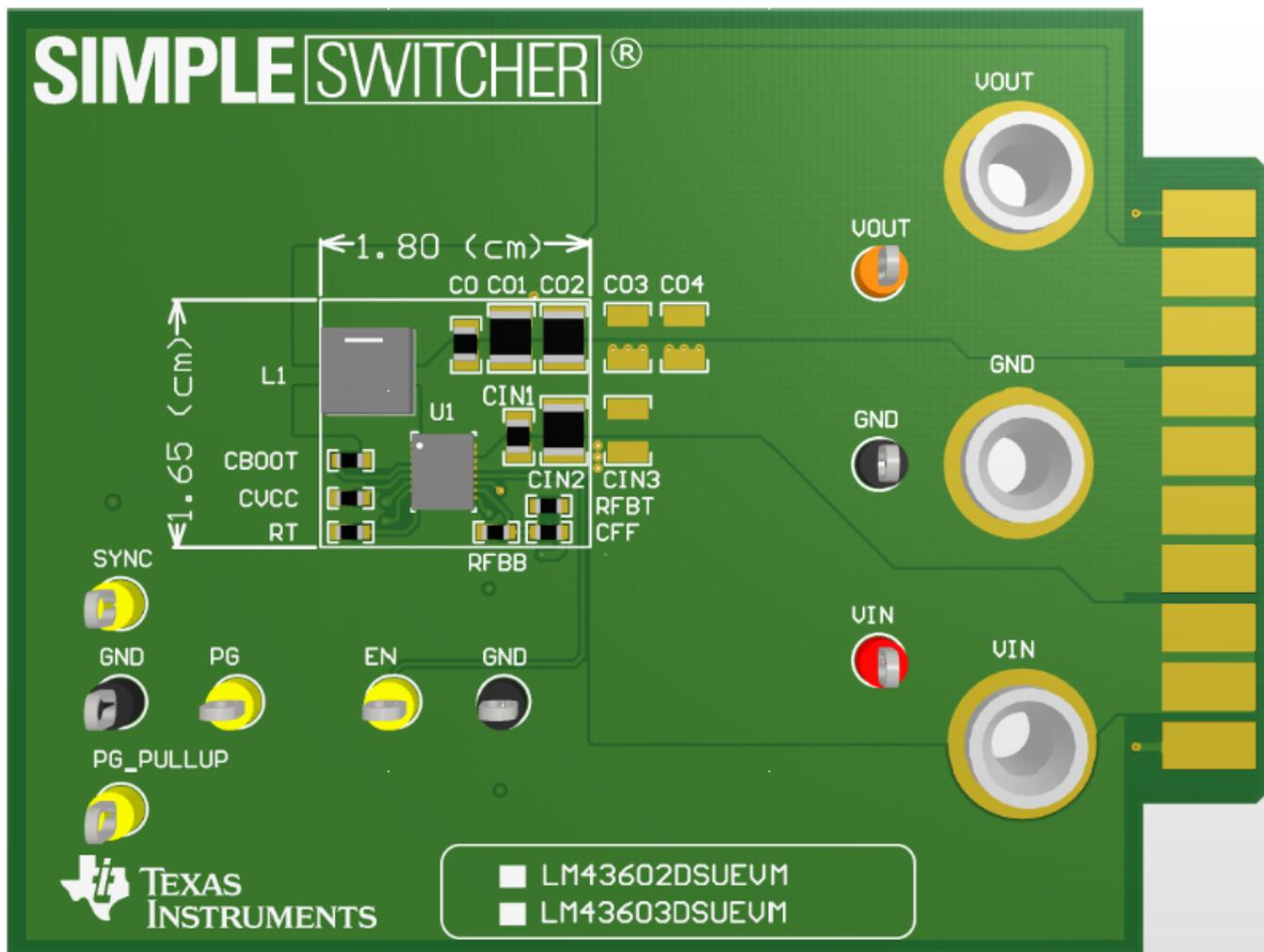
**Figure 1. Top View of LM43603DSUEVM**
