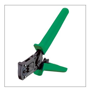
Manual tongs for termination of crimp contacts for circular connectors, with contact positioning device
