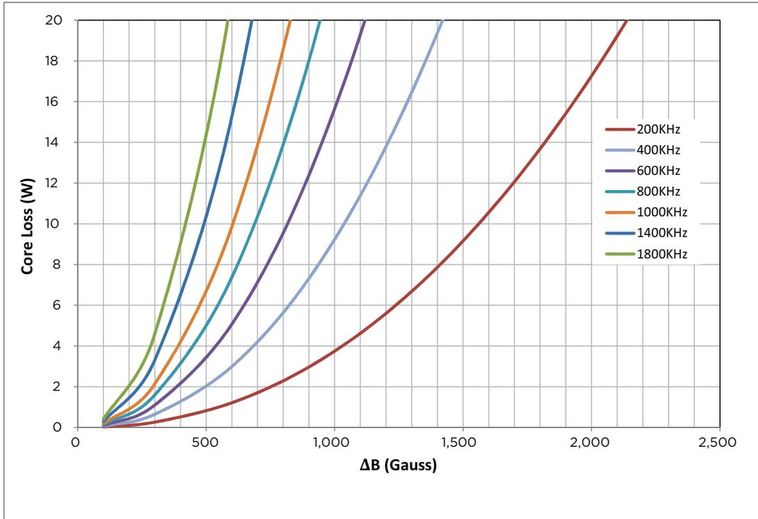
$$\Delta B \text{ (Gauss)} = K * L(\mu\text{H}) * \Delta I(\text{A})$$
