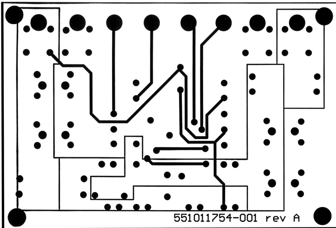
Figure 5. PCB Bottom Layer and Internal Power Plane
