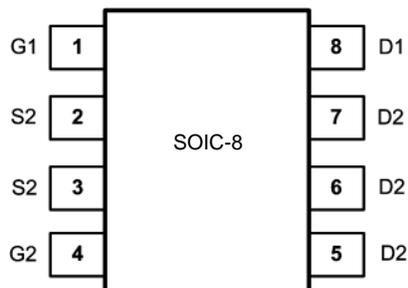
Figure 1. Pinout for Dual FET for Footprint Q3
