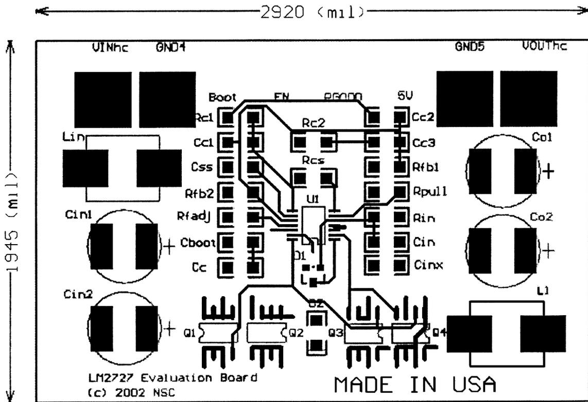
Figure 4. PCB Top Layer and Top Overlay
