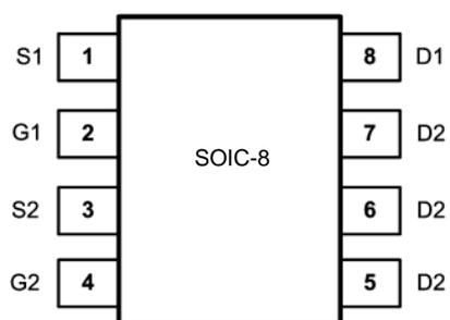
Figure 2. Pinout for Dual FET for Footprint Q4
