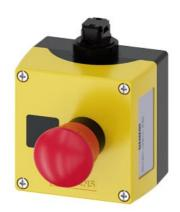
AS-Interface enclosure for command devices, 22 mm, round, Enclosure material plastic, Enclosure top part yellow, 1 control point plastic, Recess for label, A=EMERGENCY STOP mushroom pushbutton red, 40 mm, rotate-to-unlatch, 1 NC, 1 NC, spring-type terminal, floor mounting, Insulation displacement system on top, Label enclosed
