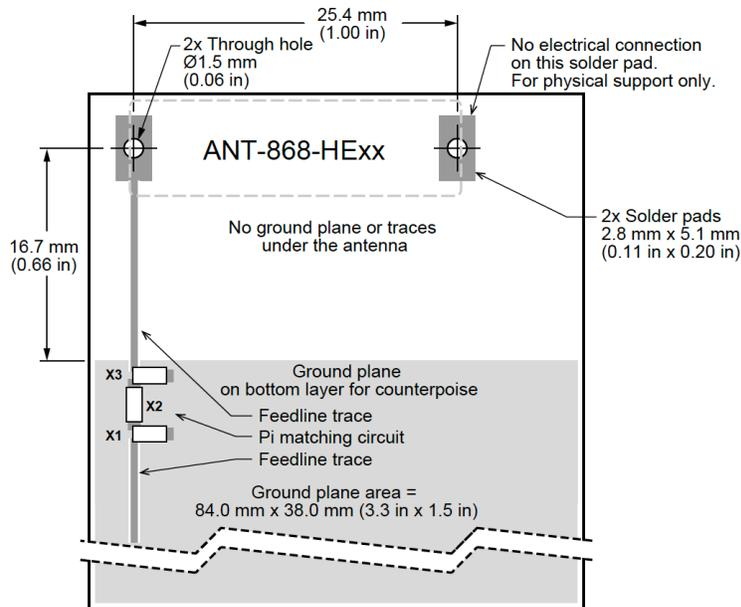
Figure 11. 868-HE Series Antenna Placement on PCB.
