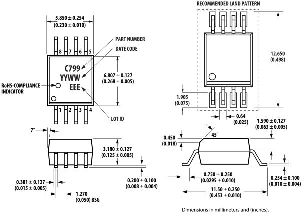
Notes: Lead coplanarity = 0.1 mm (0.004 inches). Floating lead protrusion = 0.25 mm (10 mils) max.
