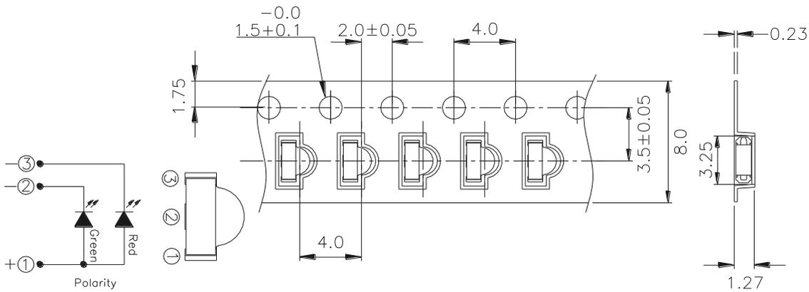
Note: The tolerances unless mentioned is  $\pm 0.1\text{mm}$ , Unit = mm
