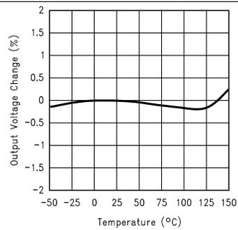
Figure 4. Percent Change in Output Voltage vs Temperature
