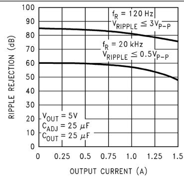
Figure 8. Ripple Rejection vs Output Current (LM1086-ADJ)
