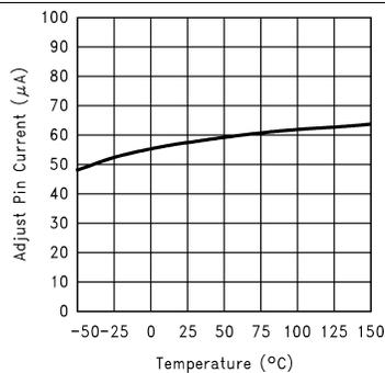
Figure 5. Adjust Pin Current vs Temperature
