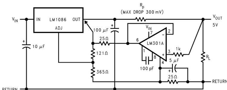
Figure 28. Remote Sensing
