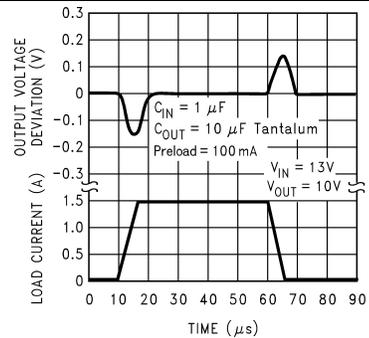
Figure 12. Load Transient Response
