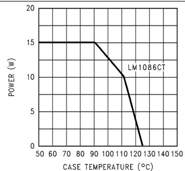
Figure 6. Maximum Power Dissipation vs Temperature
