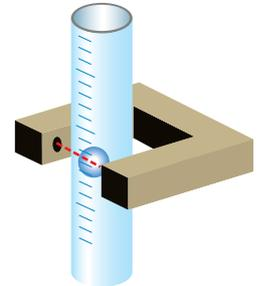
Can detect whether greater or less than set flow rate. The flow condition can be controlled all the time.
