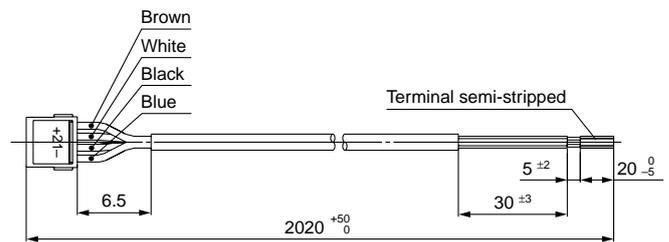
Cable Specifications of Lead Wire
