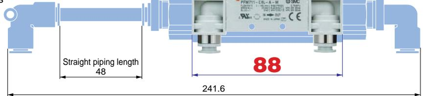
Comparison with the conventional model PF2A711 (10 to 100 ℓ/min) when  $\phi 6$  one-touch fittings are attached.
