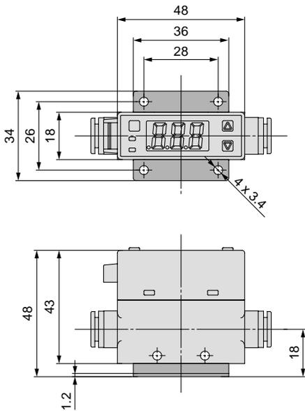
With bracket / With flow adjustment valve
