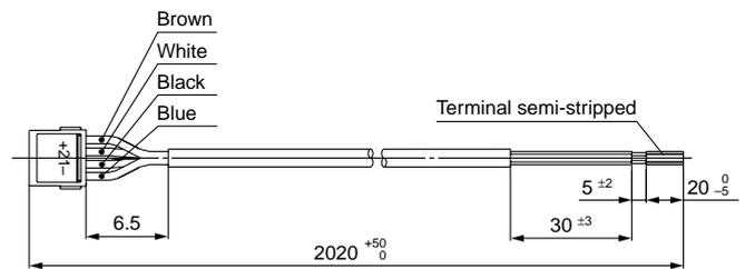
Cable Specifications of Lead Wire with Connector
