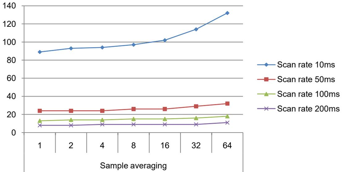
**Figure 32-8. Power Consumption [ $\mu$ A]**
