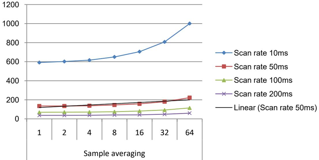
**Figure 32-10. Power Consumption [ $\mu$ A]**
