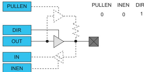
**Figure 21-7. I/O Configuration - Totem-Pole Output with Enabled Input**
