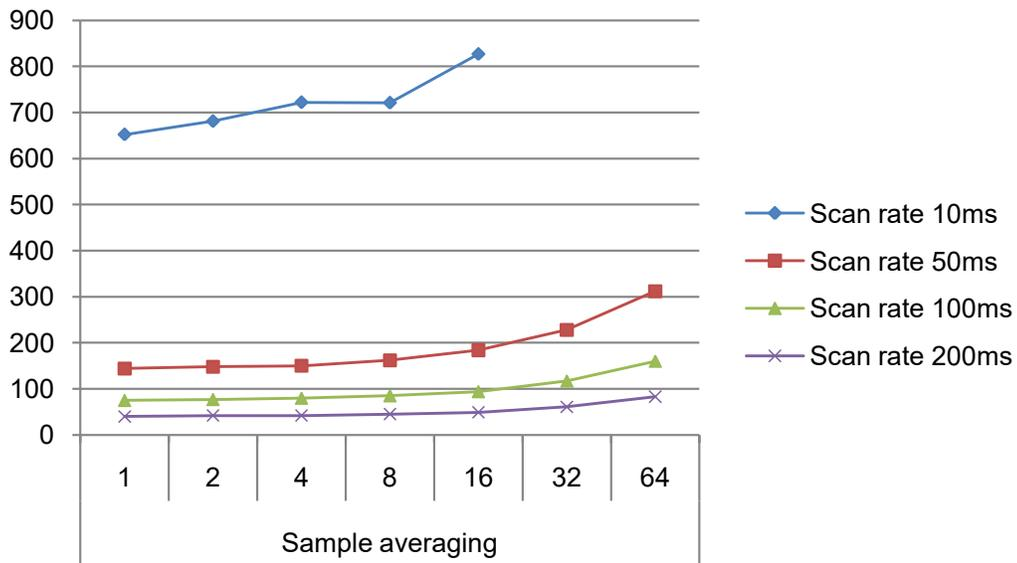
**Figure 32-11. Power Consumption [ $\mu$ A]**
