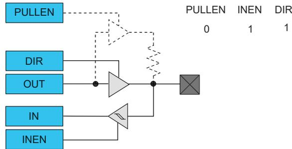
**Figure 21-8. I/O Configuration - Output with Pull**
