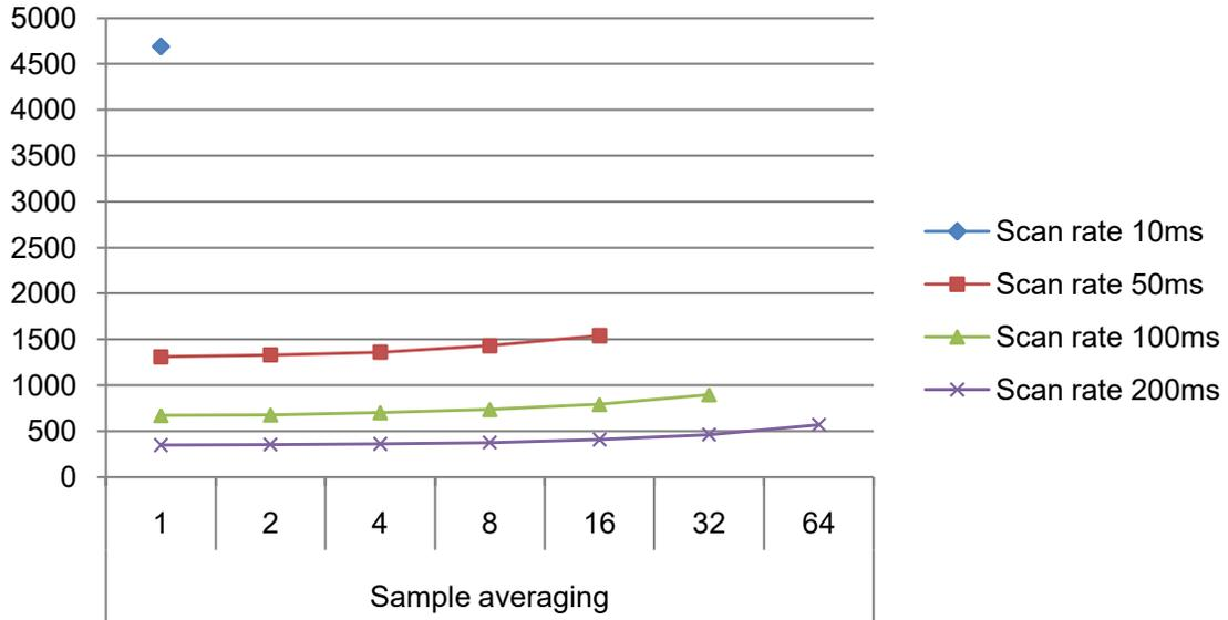
**Figure 32-12. Power Consumption [ $\mu$ A]**
