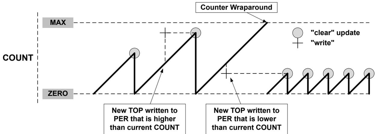
**Figure 27-8. Changing the Top Value with Down-Counting Operation**
