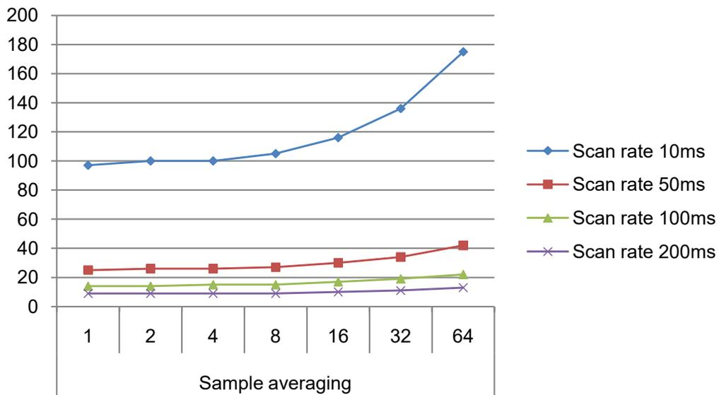
**Figure 32-9. Power Consumption [ $\mu$ A]**
