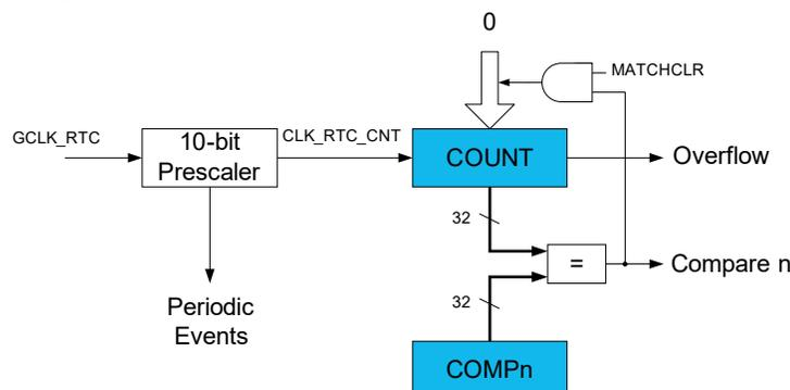
**Figure 18-2. RTC Block Diagram (Mode 1 — 16-Bit Counter)**
