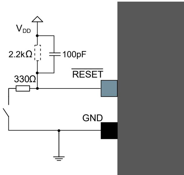
**Figure 36-5. External Reset Circuit Schematic (EFT Immunity Enhancement)**
