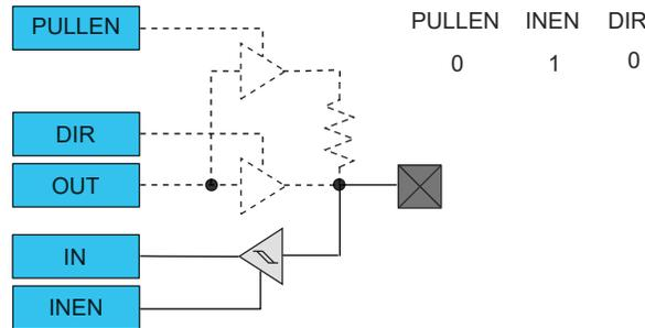
**Figure 21-5. I/O Configuration - Input with Pull**
