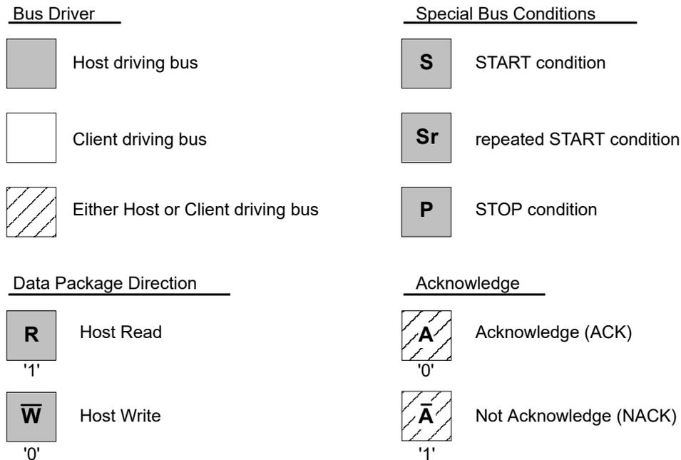
**Figure 26-3. Basic I<sup>2</sup>C Transaction Diagram**
