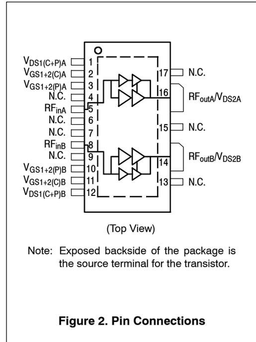
Figure 2. Pin Connections
