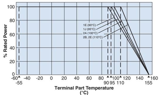
For resistors operated at a terminal part temperature of described for each size or above, a power rating shall be derated in accordance with derating curve. Please refer to "Introduction of the derating curves based on the terminal part temperature" in the beginning of our catalog before use.
