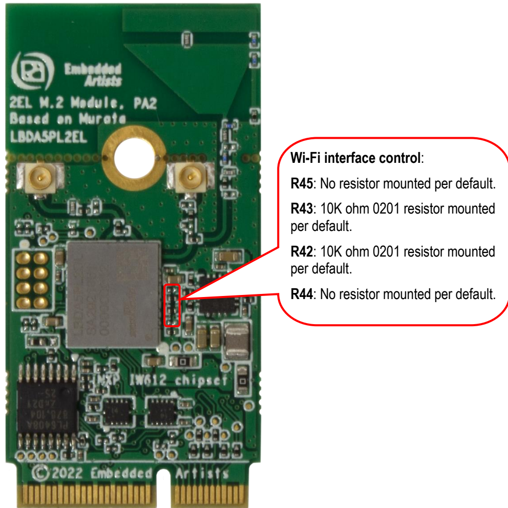
Figure 6 – 2EL/2DL M.2 Module Wi-Fi Interface Control
