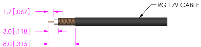
IN PROCESS 1 STRIP CABLE AND TIN INNER CONDUCTOR
