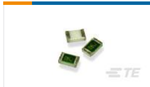
TE Part #2-1879216-7 CPF 0402 95K3 0.1% 25PPM 1K RL
