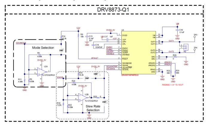
Figure 3. Mode and Slew Rate Selection Circuitry of Hardware variation
