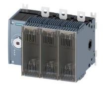
Switch disconnector with fuse 250 A, Size 3, 3-pole for LV HRC fuse Sz. 0 and 1 Front operating mechanism left Basic unit without handle flat terminal
