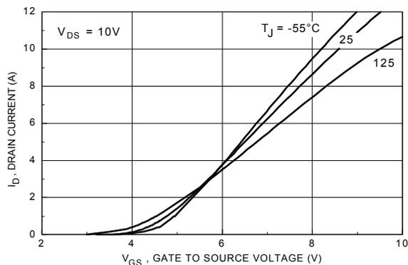
Figure 5. Transfer Characteristics.
