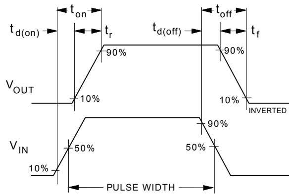
Figure 12. Switching Waveforms
