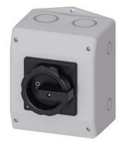
SENTRON, Switch disconnector 3LD, main switch, 4-pole, 63 A, Operating power at AC- 23 A at 400 V: 22 kW, molded-plastic encapsulation for metric cable gland, rotary operating mechanism, black
