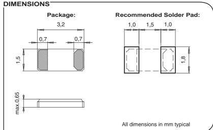
Miniature SMT ceramic package with metal lid Low package height 0.65 mm max. SMD-package in Tape and Reel Ind. and Ext. temperature ranges AEC-Q200 automotive compliant High stability, Low aging Low power consumption High shock and vibration resistance
