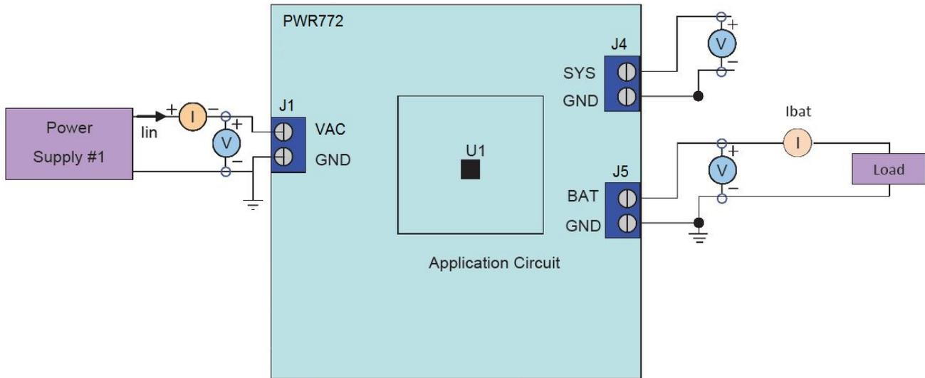
Figure 1. Original Test Setup for bq25606 EVM
