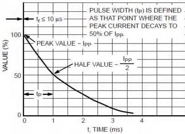
Figure 6. Pulse Waveform
