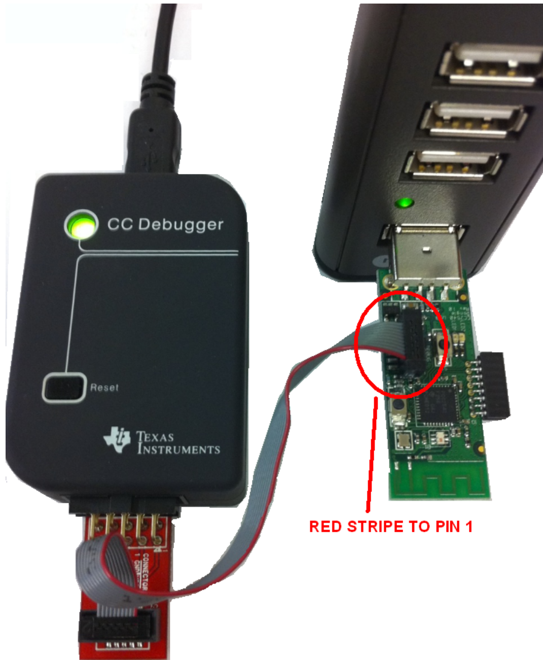
Figure 6-2. CC2540 USB Dongle Connected to CC Debugger
