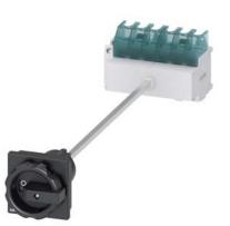
SENTRON, Switch disconnector 3LD, main switch, 6-pole, lu: 25 A, Operating power / at AC-23 A at 400 V: 9.5 kW, floor mounting with door coupling, 1 NC, 1 NO, rotary operating mechanism, black, 4-hole mounting of the handle
