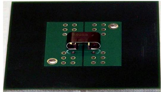
In contrast to the flat chip format, the OARS format keeps the hot spot thermally distant from the solder joints and reduces undesirable heat delivery into the PCB. Further thermal images for other ohmic values and power dissipations are available on request.
