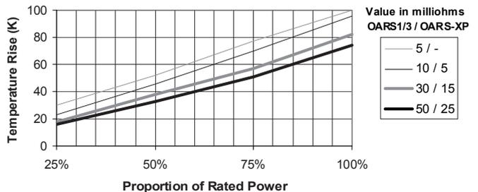
Note: Temperature rise data are given here for typical mounting conditions. Actual figures depend on PCB copper weight, mounting pad size, track width and substrate type. Also, the open air format responds better to forced air cooling than chip format resistors. For values below 5 milliohms allowance should be made for heat generated in the copper tracks themselves. Application-specific guidance is available on request.
