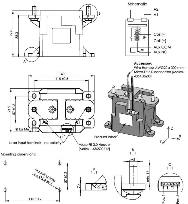
In case of no tolerance shown in dimensional drawing, general tolerances apply: dimension  $\leq$  10 mm:  $\pm$  0.3 mm; dimension 10 to 50 mm:  $\pm$  0.6 mm; dimension > 50 mm:  $\pm$  1 mm.
