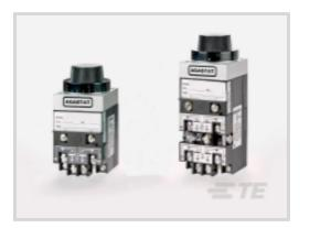
Type of Control: Knob Input Voltage: 125 VDC Contact Current Rating: 10 A Mode of Operation: On-Delay Delay Time: 1.5 – 15 seconds
