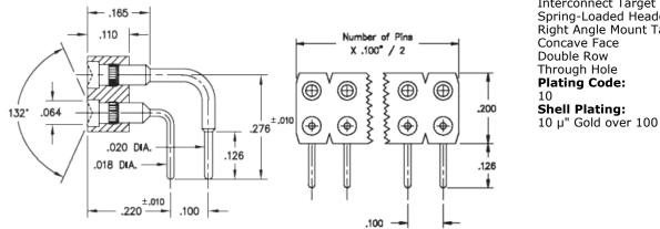
**Description:** Interconnect Target Connector Spring-Loaded Header Right Angle Mount Target with
