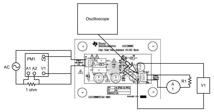
Figure 2. Test Setup
