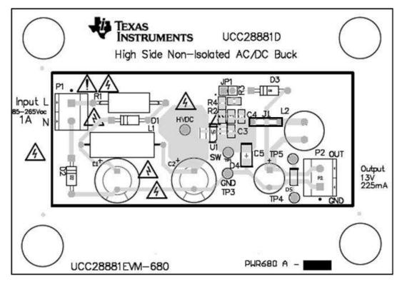
Figure 16. UCC28881EVM-680 Assembly Drawing/Layout
