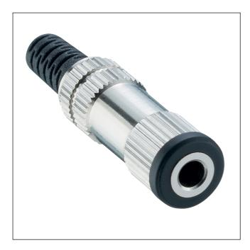
Jack socket acc. to JIS C 6560 JC35J2A, 3.5 mm, 2 poles/ mono, straight version, with metal housing, bend protection and solder terminals
