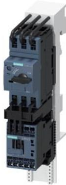
Load feeder fuseless, Direct-on-line starting 400 V AC, Size S00 0.22...0.32 A 230 V AC Spring-type terminal for 60 mm busbar systems (also fulfills type of coordination 1) Type of coordination 2, I<sub>q</sub> = 150 kA 1 NO (contactor)
