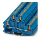
Double-level terminal block, nom. voltage: 800 V, nominal current: 22 A, connection method: Push-in connection, 1st and 2nd level, Rated cross section:  $2.5~\text{mm}^2$ , cross section:  $0.14~\text{mm}^2$  -  $4~\text{mm}^2$ , mounting type: NS 35/7,5, NS 35/15, color: blue
