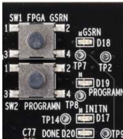
Figure 3. ECP5 Status LEDs and Push-button Controls
