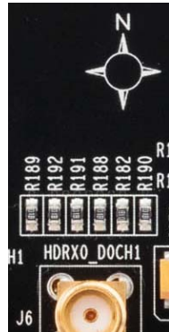
Figure 20. CFG[2:0] Setting Resistor Field – Revision A
