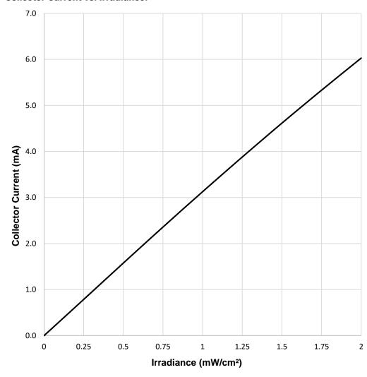
Testcondition:  $Ee = 0.5 \text{ mW/cm}^2$ , VCE = 5 V
