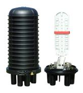
FOSC<sup>™</sup>400 A4 Fiber Optic Splice Closure, Heat Shrink Cable sealing, one pre-installed 24-splice tray, cable blocking, ground feedthrough lugs, with test valve
