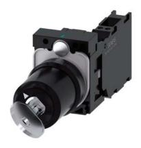
key-operated switch Siemens, 22 mm, round, plastic, lock number SSG10, with 2 keys, 2 switch positions O-I, latching, 10:30h/13:30h, key removal O+I, with holder, 1 NO+1 NC, spring-loaded terminal, with laser labeling, inscription or symbol customer-specific selection with SIRIUS ACT configurator (CIN)
