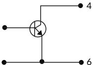
Positive logic: "On" if pin 4 is high >3.5V to 160VDC
