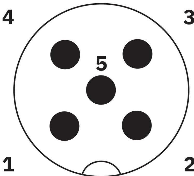
Coolant tank fill-level sensor connected via M12 male with A-coding
