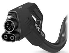
CHARX connect professional, HPC DC charging cable, with cooled vehicle charging connector and cooled cable, for charging electric vehicles (EV) with direct current (DC), with charging connector holder, with replaceable mating face frame, without panel feed-through, Single-core wires for four-conductor measurement are not connected and are non-functional, CCS type 1, SAE J1772, IEC 62196-3-1, 500 A / 1000 V (DC), PHOENIX CONTACT logo, cable: 5 m, black, straight
