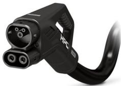
CHARX connect professional, HPC DC charging cable, with cooled vehicle charging connector and cooled cable, for charging electric vehicles (EV) with direct current (DC), with replaceable mating face frame, with replaceable DC power contacts, without panel feed-through, Single-core wires for four-conductor measurement are not connected and are non-functional, CCS type 2, IEC 62196-3-1, 500 A / 1000 V (DC), PHOENIX CONTACT logo, cable: 5 m, black, straight
