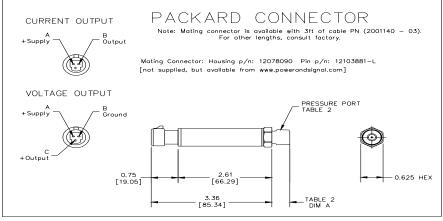
TABLE 1 TABLE 2 CONNECTION PRESSURE PORT DIM A CODE CONNECTOR CABLE 2 FOOT 0.45 [11.43] 7/16-20 MALE 0-RING 0.33 [8.38] CABLE 4 FOOT 1/4 NPT 0.50 [12.7] 3 CABLE 10 FOOT 5 PACKARD CONNECTOR 6 1/8 NPT 0.475 [12.07]
