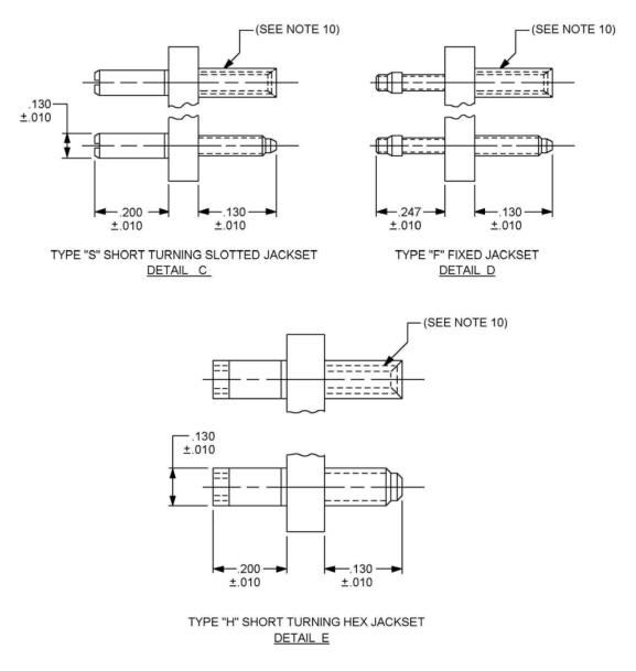
FIGURE 1. Connectors, plug, .100 (2.54 mm) spacing - Continued.
