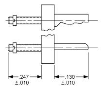
TYPE "Y" (D-SHAPED) GUIDE PIN AND SOCKET <u>DETAIL H</u>
