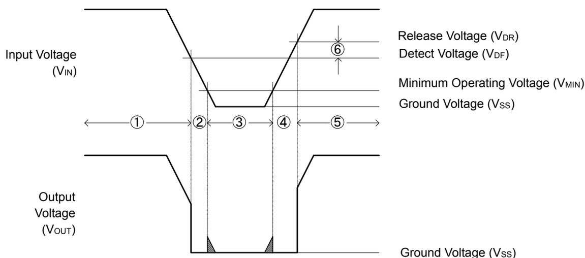
Note: For explaining in a simplified case, an operation time of the circuit is not counted.
