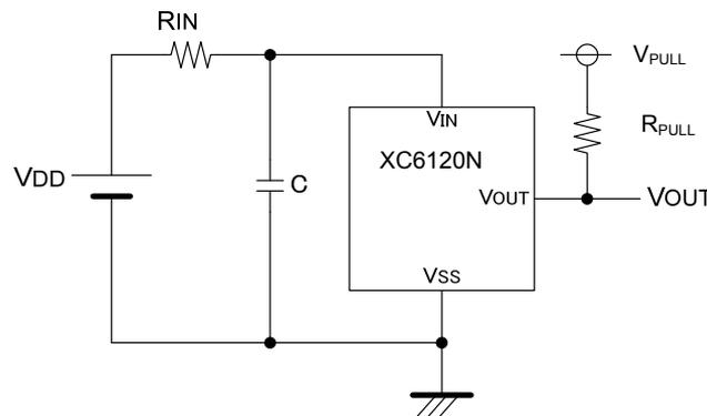
[Figure 1: Circuit connected with the input resistor]
