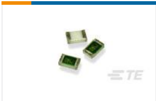
TE Part #5-1879215-7 CPF 0402 17K4 0.1% 25PPM 1K RL
