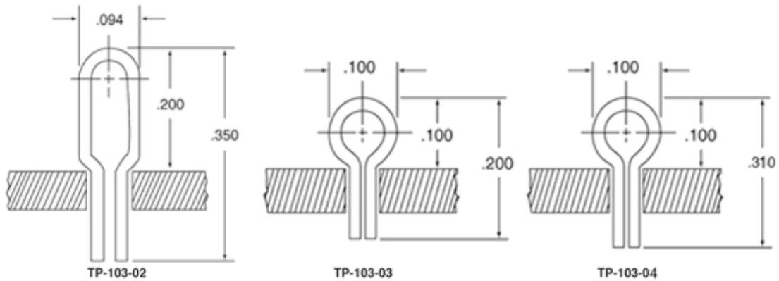
\*Note: Leads flared to provide retention in the printed circuit board.
