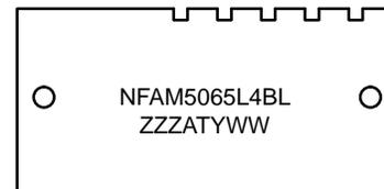
Device marking is on package top side
